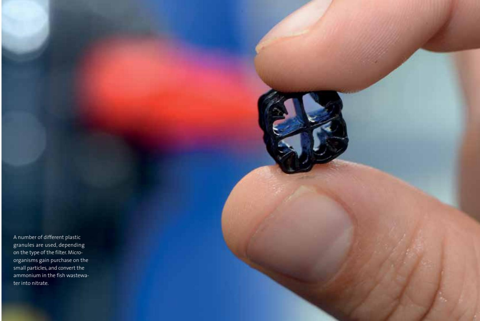
of a biofilter colonized by microorganisms. They live on “trickling filters”, which are bits of plastic with large surface areas. The bacteria convert the ammonium into nitrate through a process called nitrification. Nitrate is an excellent fertilizer, which accelerates the growth of the tomato plants.
