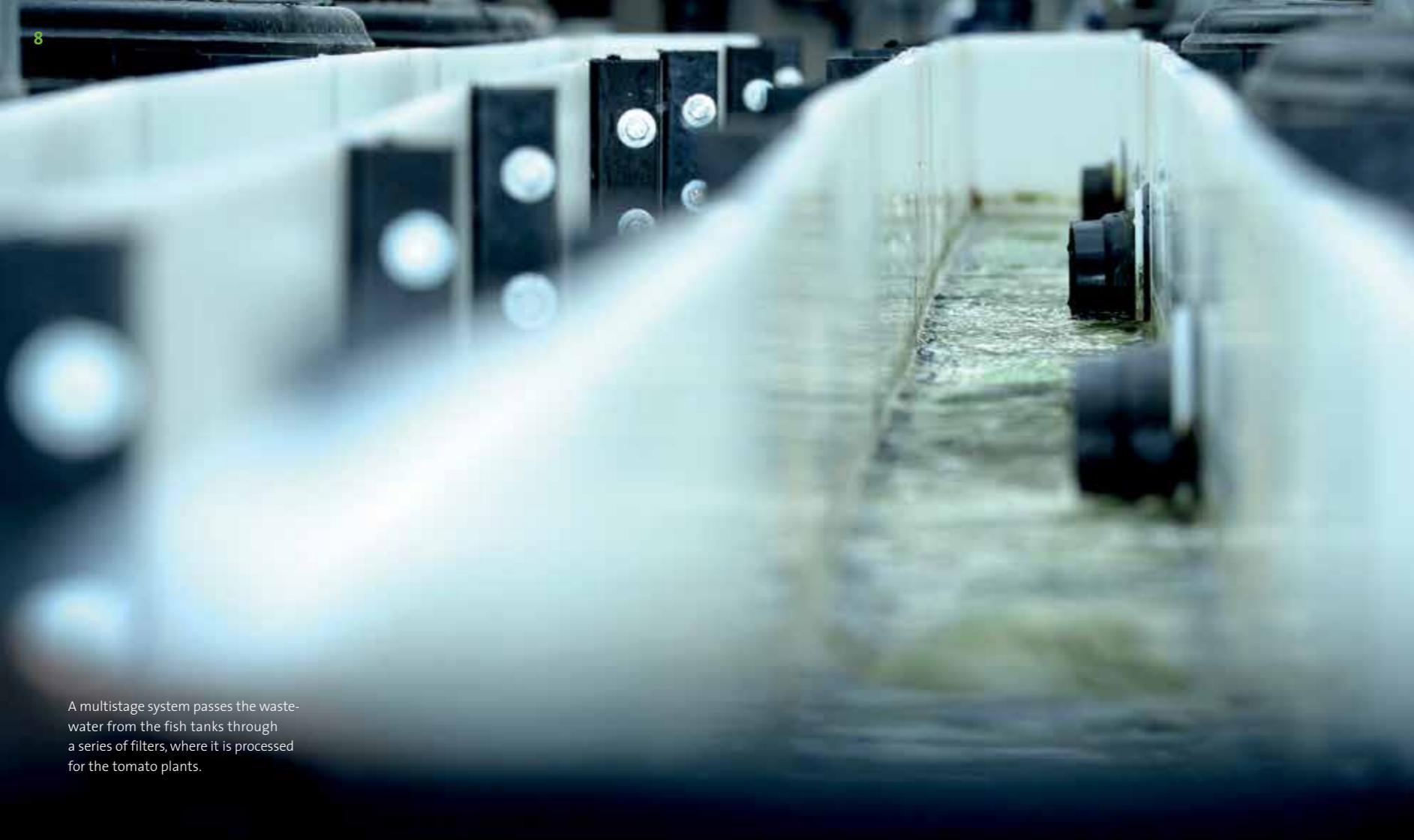
A multistage system passes the wastewater from the fish tanks through a series of filters, where it is processed for the tomato plants.
